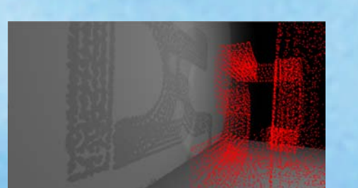
Figure 3: After blurring the depth map, the output is smoother and more representative of a surface.
